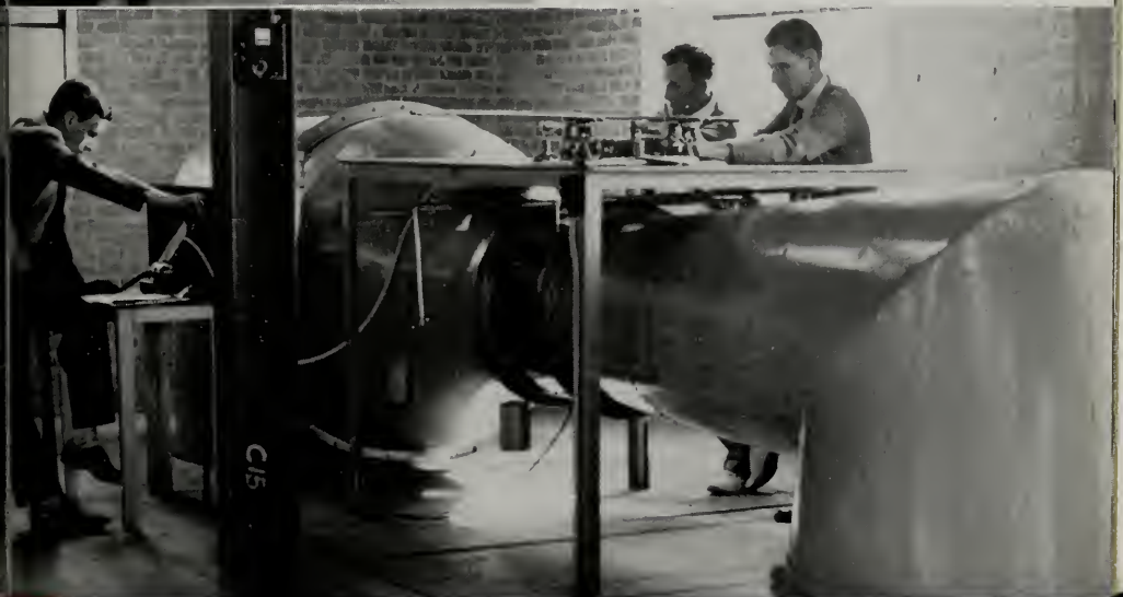
Below: Wind tunnel for studying characteristics of air-foil shapes.
